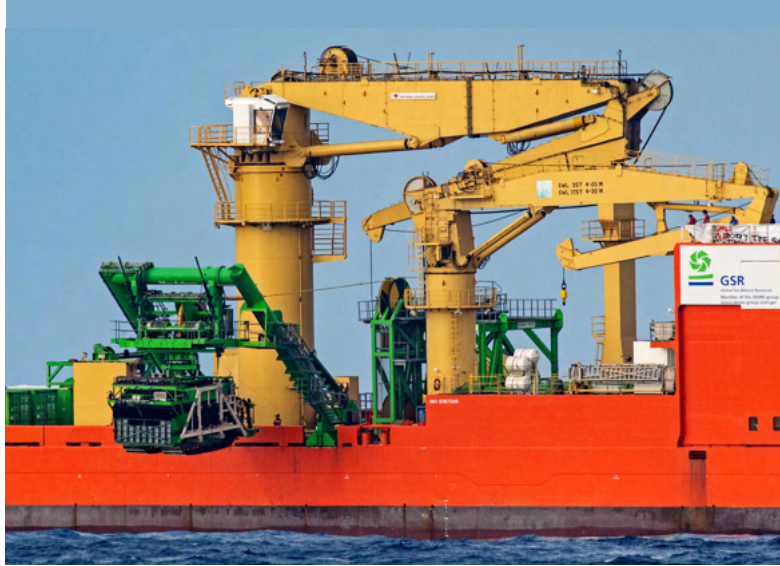
THE PATANIA II NODULE COLLECTOR IS LAUNCHED FROM MARINE VESSEL NORMAND ENERGY, DOCUMENTED FROM THE RAINBOW WARRIOR IN THE PACIFIC. © MARTEN VAN DIJL / GREENPEACE
